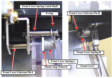
Figure 4-23. Front Cover Removal
