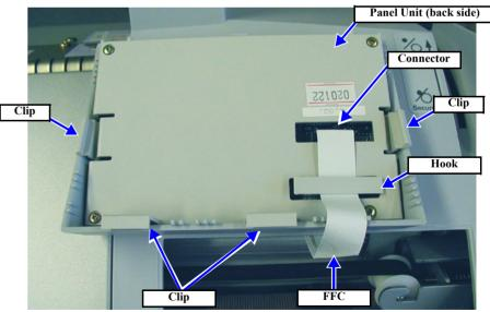
Figure 4-5. Panel Unit Removal 2/2
