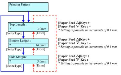
Figure 5-34. Menu Transition for Top & Bottom Adjustment
