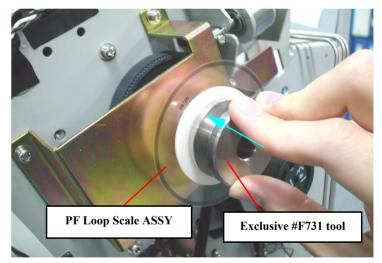
Figure 4-56. Affixing the PF Loop Scale ASSY
