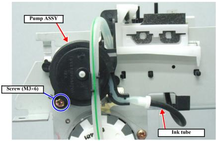
Figure 4-77. Removing the Pump ASSY 2/2
