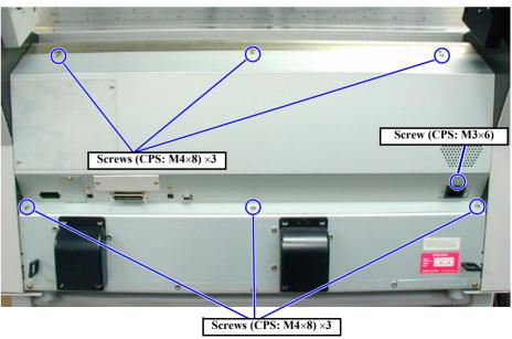
Figure 4-17. Rear Cover Removal 2/2
