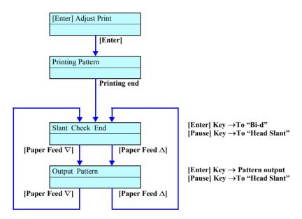
Figure 5-42. Menu Transition of Head Slant
