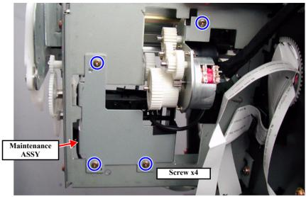
Figure 4-72. Removing the Maintenance ASSY
