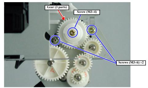
Figure 4-76. Removing the Pump ASSY 1/2
