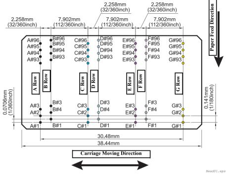
Figure 2-3. Nozzle Arrangement
