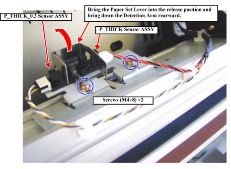
Figure 4-59. P\_THICK and P\_THICK\_0.3 Sensors Removal
