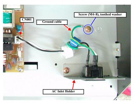
Figure 4-81. Removing the AC Inlet Holder
