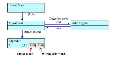
Figure 5-19. Menu Transition for Edge AD Adjustment
