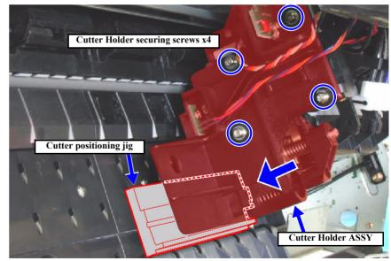
Figure 5-74. Cutter Holder ASSY height adjustment
