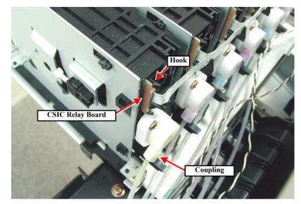
Figure 4-67. CSIC Relay Board Removal
