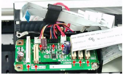
Figure 4-31. CR Board Connectors Disconnection
