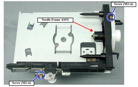
Figure 4-69. Disassembling the Ink Holder ASSY 1/2
