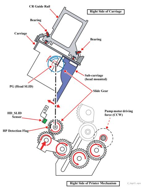
Figure 2-4. Carriage Mechanical Unit and PG Adjustment Unit
