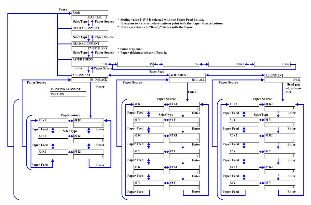
Figure 1-18. Level Structure of Gap Adjustment Menu
