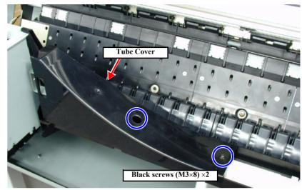
Figure 4-63. Ink Tube Cover Removal
