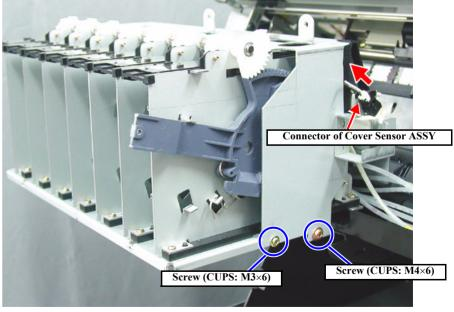
Figure 4-64. I/H Frame Removal 1/2
