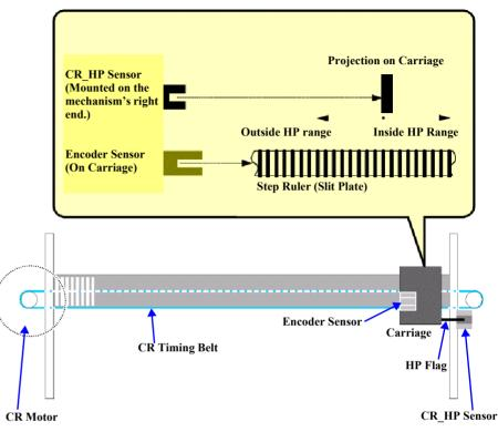
Figure 2-2. Carriage Mechanism Unit, Carriage Moving Unit
