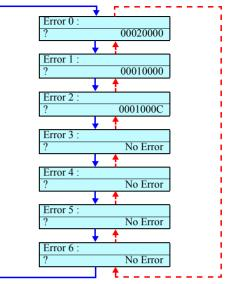
Figure 5-11. Menu Transition of Record of Errors
