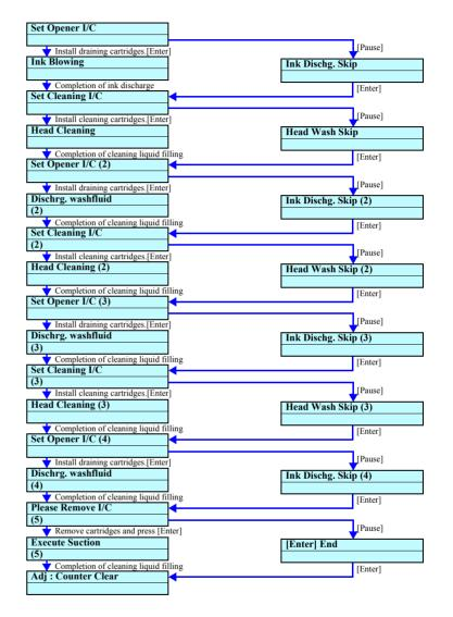
Figure 5-57. Menu Transition for Head Cleaning
