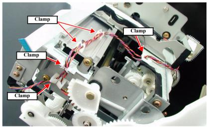
Figure 4-45. Releasing the HEAD\_SLIDE Sensor ASSY Harness
