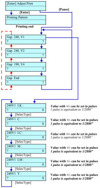
Figure 5-54. Menu Transition for Uni-D Adjustment
