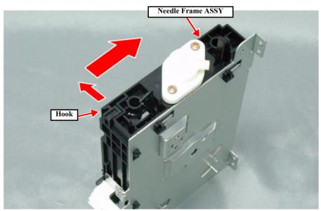
Figure 4-70. Disassembling the Ink Holder ASSY 2/2
