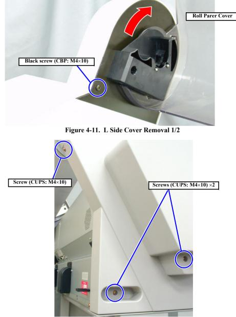
Figure 4-12. L Side Cover Removal 2/2
