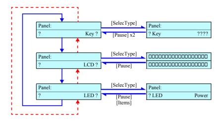
Figure 5-5. Menu Transition of Panel Test
