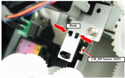
Figure 4-47. Removing the CR\_HP Sensor
