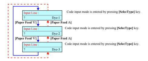
Figure 5-23. Menu Transition for Input Line Selection
