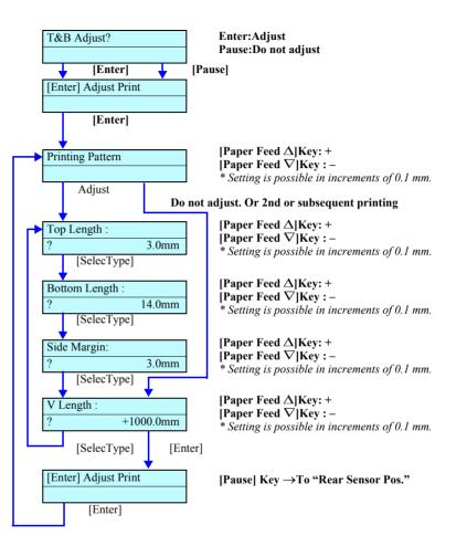
Figure 5-32. Menu Transition for Feed Correction +T&B Adjustment
