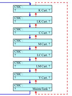
Figure 5-12. Menu Transition for Cartridge Selection
