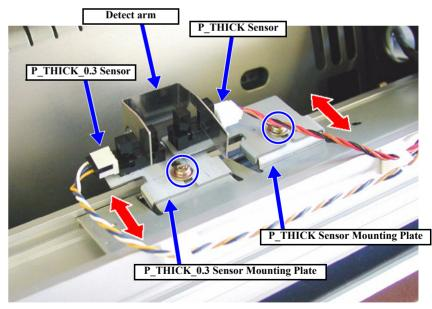
Figure 5-67. P\_THICK Sensor / P\_THICK\_0.3 Sensor Position Adjustment
