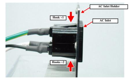
Figure 4-82. Removing the AC Inlet
