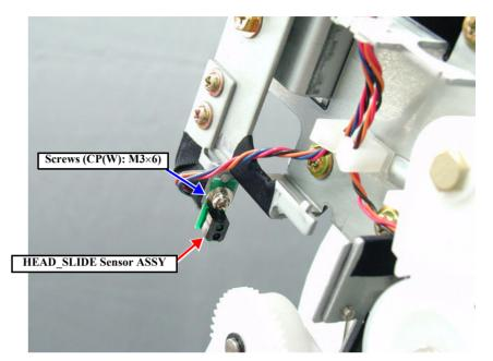
Figure 4-44. Removing the HEAD\_SLIDE Sensor ASSY
