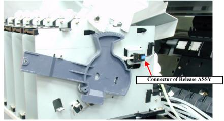
Figure 4-66. Release Sensor (I/H Lever) Removal
