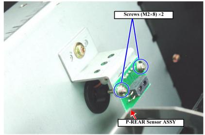
Figure 4-61. Removing the P\_REAR Sensor ASSY
