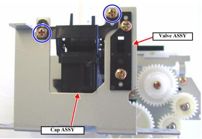
Figure 4-75. Removing the Cap ASSY
