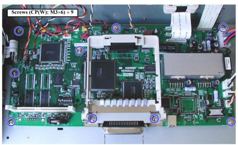
Figure 4-83. C472MAIN Board Removal
