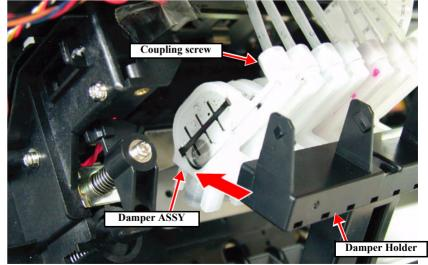
Figure 4-29. Damper ASSY Removal
