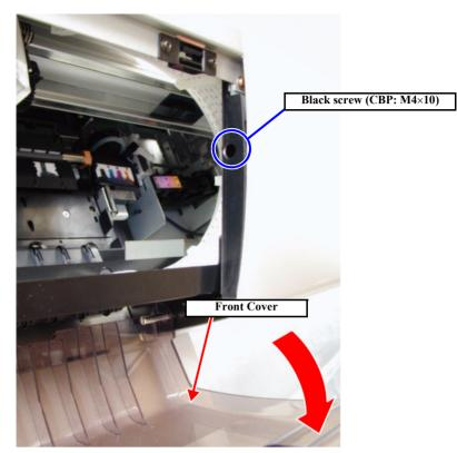
Figure 4-9. R Side Cover Removal 4/5
