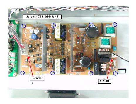
Figure 4-80. Power Supply Board Removal
