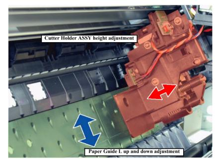
Figure 5-71. Cutter Positioning Adjustment
