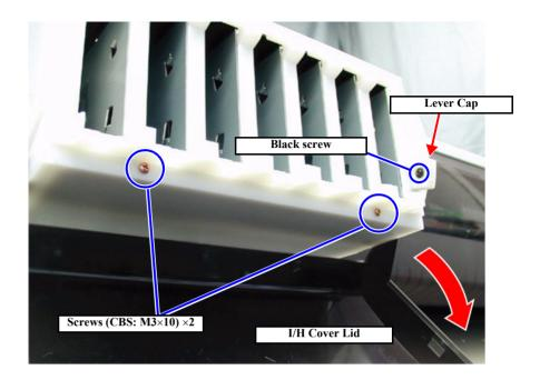
Figure 4-13. I/H Cover Removal
