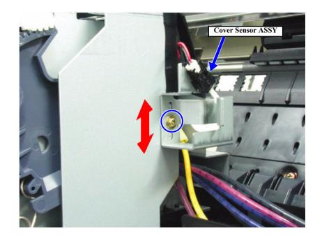
Figure 5-68. Adjusting the Cover Sensor ASSY Mounting Position
