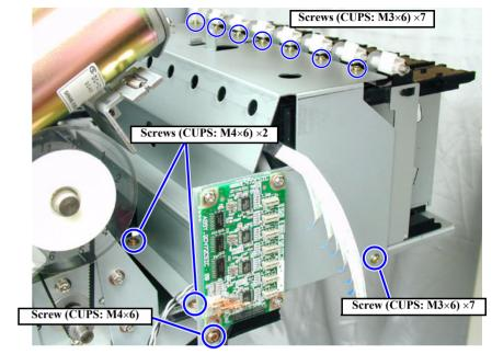
Figure 4-65. I/H Frame Removal 2/2
