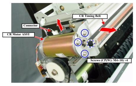
Figure 4-43. Removing the CR Motor ASSY
