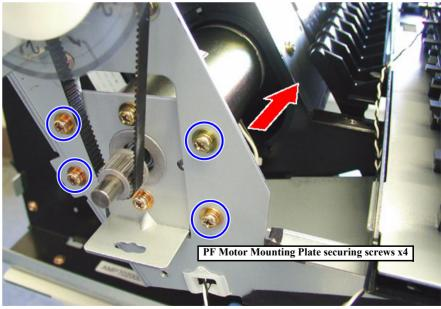
Figure 4-51. Removing the PF Motor.
