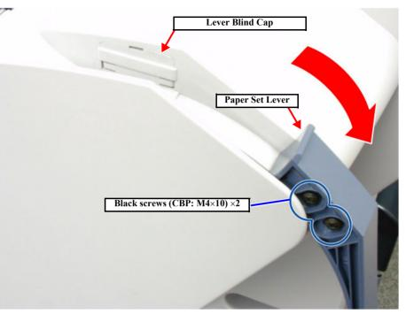
Figure 4-6. R Side Cover Removal 1/5
