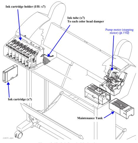
Figure 2-17. Ink Supply Mechanism
