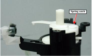
When installing the pump reduction gear, make sure that the gears are engaged properly.
