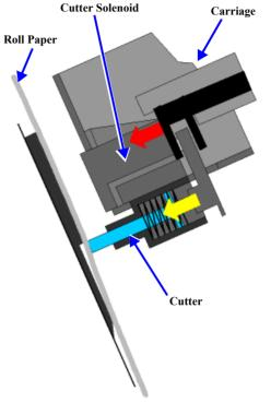
Figure 2-10. Carriage Unit Cutter Solenoid
