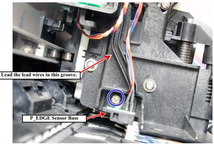
Figure 4-40. Removing the P\_EDGE Sensor ASSY 2/2
