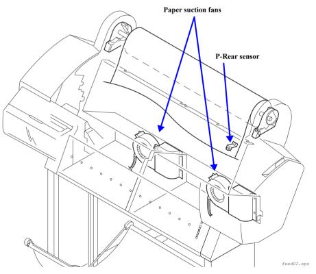
Figure 2-13. Paper Feed Mechanical Unit (Stylus Pro 7600) 2/2
