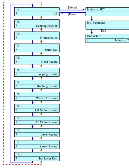
Figure 5-63. Menu Transition for Parameter Initialization
