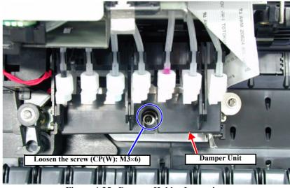
Figure 4-25. Damper Holder Loosening
