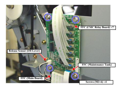
Figure 4-62. Disconnecting the C472 SUB-B Board Connectors
