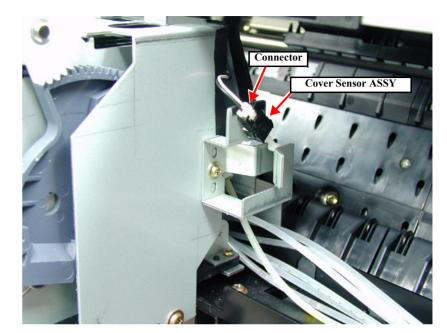
Figure 4-71. Removing the Cover Sensor ASSY
