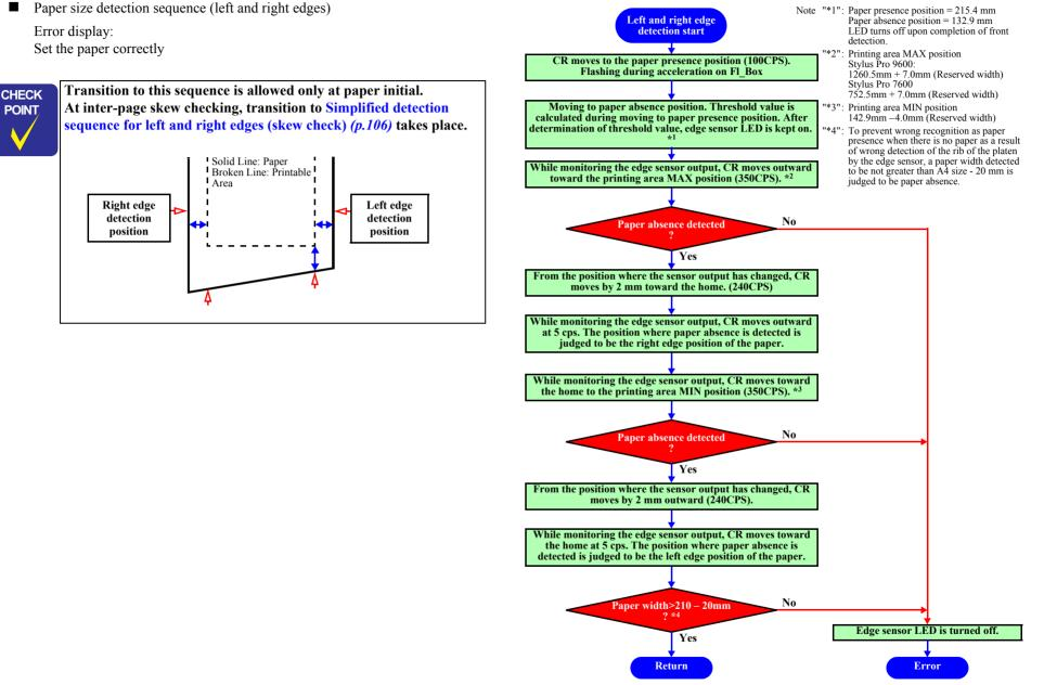
Figure 2-7. Paper Size Detection Sequence (Left and Right Edges)
