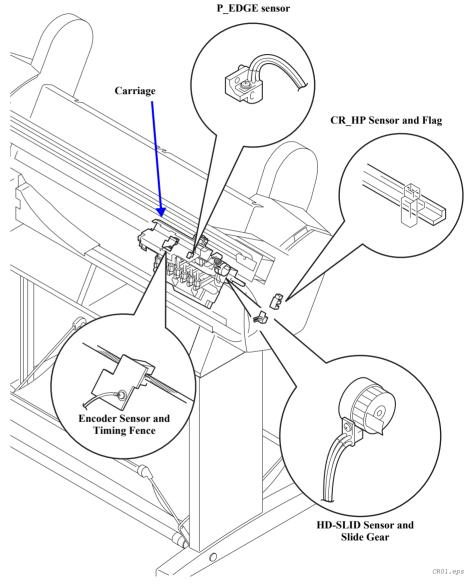
Figure 2-1. Carriage Mechanism
