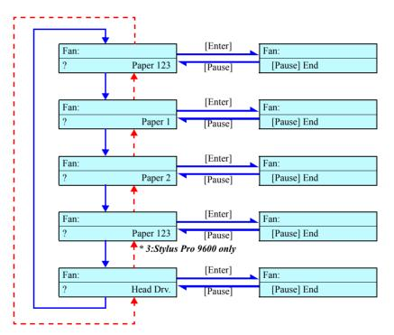
Figure 5-8. Menu Transition of Fan Test
