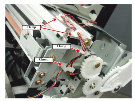
Figure 4-46. Releasing the CR\_HP Sensor ASSY Harness
