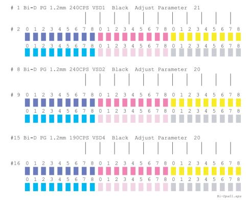
Figure 5-53. Print Patterns for Bi-D Adjustment Checking
