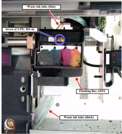
Figure 4-79. Removing the Flushing Box ASSY
