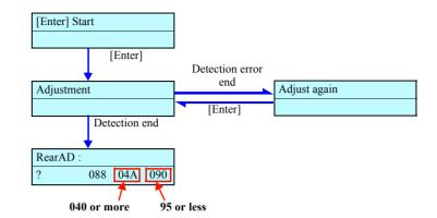
Figure 5-18. Menu Transition for Rear AD Adjustment
