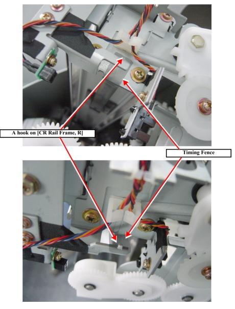
Figure 4-49. CR Encorder - Timing Fense Removal
