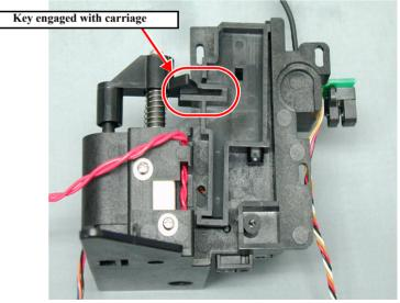
Figure 4-34. Cutter Holder ASSY (Back: Carriage Side)
