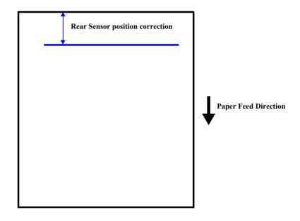
Figure 5-37. Rear Sensor Position Adjustment Pattern
