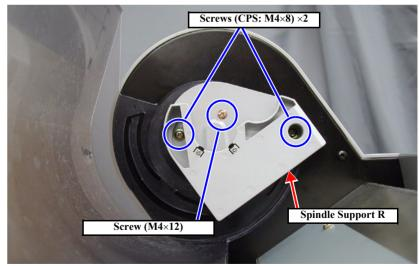
Figure 4-21. Roll Paper Cover removal
