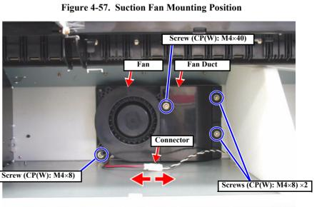
Figure 4-58. Suction Fan Removal
