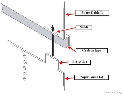
Figure 4-19. Paper Guide L2 Installation
