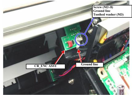
Figure 4-38. CR Encoder Sensor Removal 2/2
