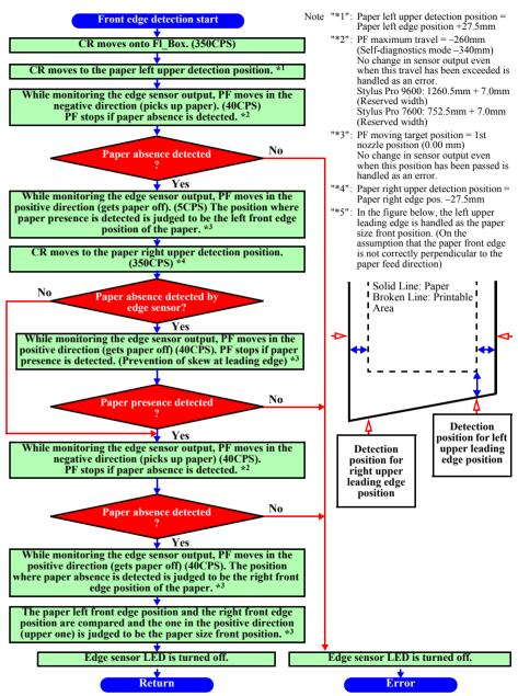
Figure 2-8. Paper Size Detection Sequence (Front Edge)
