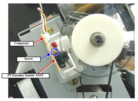
Figure 4-52. Removing the PF Encoder Sensor.
