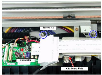
Figure 4-39. Removing the P\_EDGE Sensor ASSY 1/2
