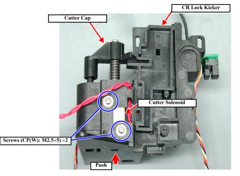
Figure 4-36. Cutter Solenoid Removal
