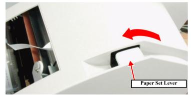
Figure 4-10. R Side Cover Removal 5/5
