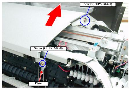
Figure 4-15. H Top Cover Removal on right side
