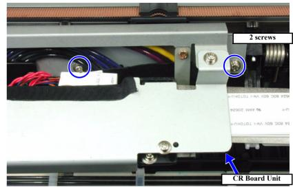
Figure 5-69. Adjusting the CR Encoder Sensor Mounting Position 1/2
