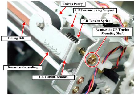
Figure 4-42. Loosening the CR Timing Belt
