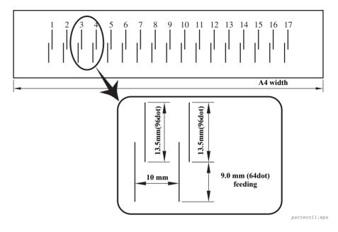
Figure 1-16. Paper Thickness Detection Pattern
