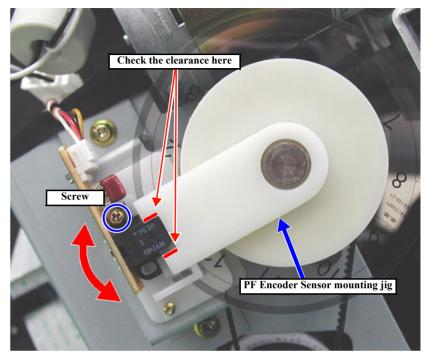
Figure 5-76. PF Encoder Sensor Installation Position Adjustment
