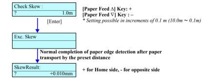
Figure 5-31. Menu Transition for Skew Checking
