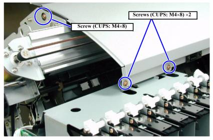
Figure 4-14. H Top Cover Removal on left side
