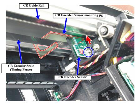
Figure 5-70. Adjusting the CR Encoder Sensor Mounting Position 2/2
