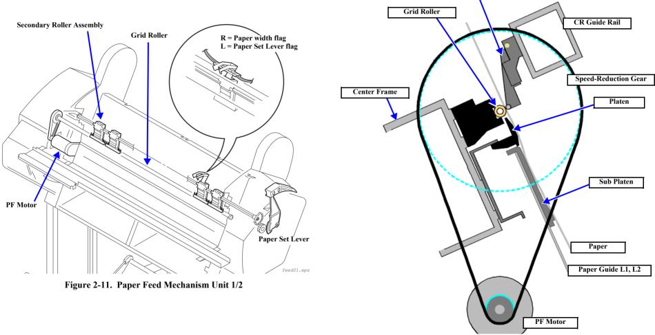
Figure 2-12. Paper Feed Mechanical Unit PF Rail Unit
