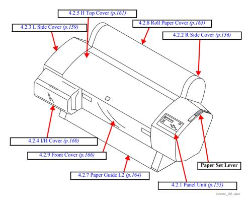
Figure 4-3. Housing Part Diagram
