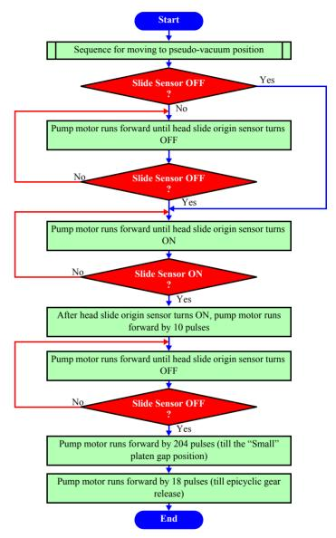
Figure 2-5. Head Slide (PG Change) Initialization Sequence
