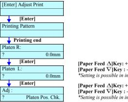
[Paper Feed  $\Delta$ ]Kev: + [Paper Feed  $\nabla$ ]Kev : – \*Setting is possible in increments of 0.1 mm.
