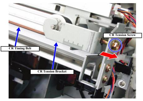
Figure 5-64. CR Timing Belt Tension Adjustment
