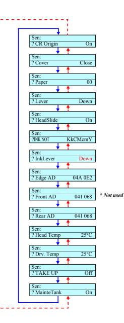
Figure 5-6. Menu Transition of Sensor Test
