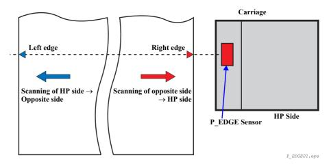
Figure 2-6. Carriage Unit Paper Width Detection Sensor
