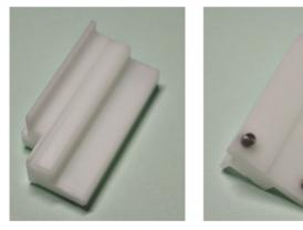
The positions where to set the jig for checking and adjustment should be the right and left ends as close to the frame as possible.
