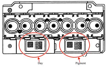
Figure 5-24. Head Code Label Position
