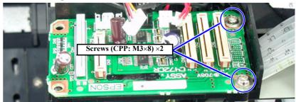
Figure 4-32. CR Board Removal
