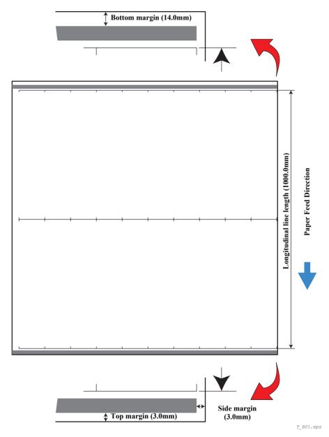
Figure 5-33. Print Pattern for Feed Correction + T&B Adjustment
