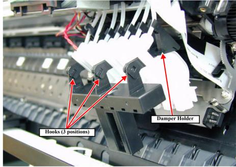
Figure 4-28. Damper Holder Removal
