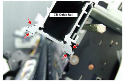
Figure 6-1. Lubricating Positions on the CR Guide Rail
