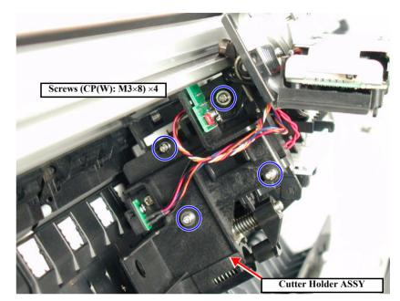
Figure 4-33. Removing the Cutter Housing
