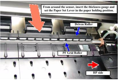
Figure 5-66. Gauge Setting Position
