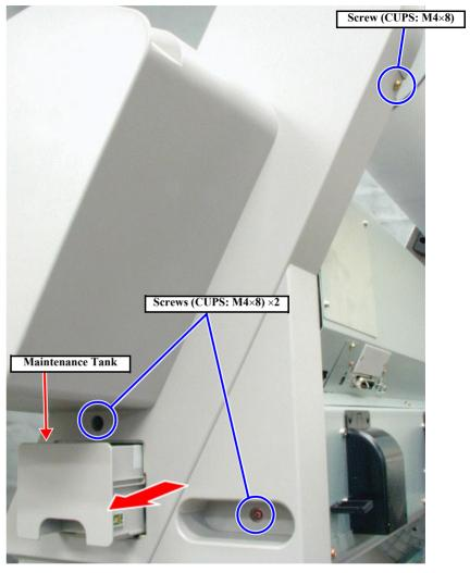
Figure 4-8. R Side Cover Removal 3/5
