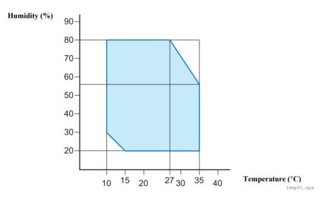
Figure 1-2. Environmental Conditions: Temperature/Humidity
