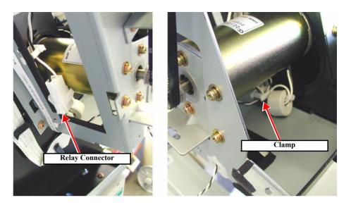
Figure 4-50. Removing the PF Motor ASSY Harness Connector.
