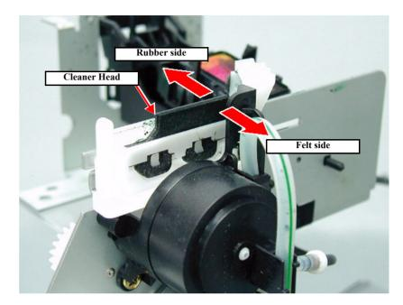
Figure 4-78. Removing the Cleaner Head
