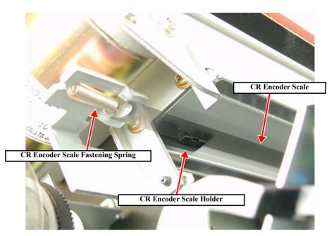
Figure 4-48. Releasing from the CR Encoder Scale Fastening Spring
