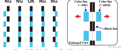
Figure 5-55. Print Pattern (Head Gap Adjustment)
