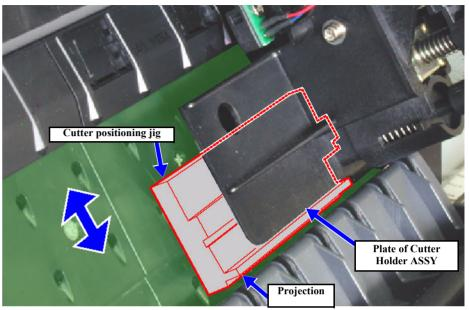
Figure 5-73. Paper Guide L up and down adjustment
