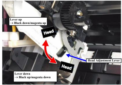
Figure 5-46. Head Slant Adjustment 2/2
