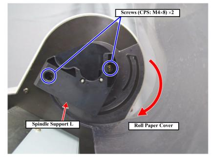
Figure 4-20. Roll Paper Cover removal
