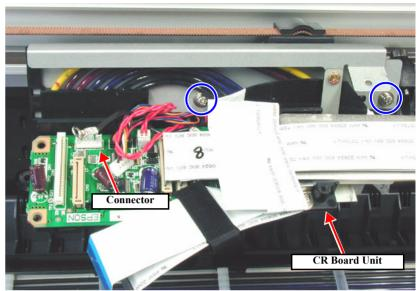
Figure 4-37. CR Encoder Sensor Removal 1/2
