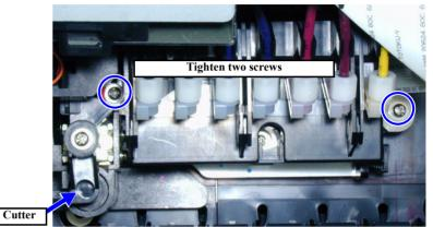
Figure 5-45. Head Slant Adjustment 1/2
