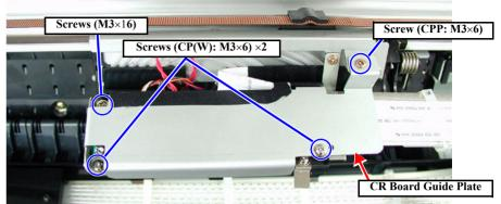
Figure 4-30. CR Board Guide Removal
