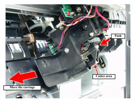
Figure 4-24. Carriage Lock Release
