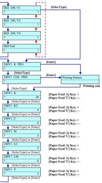
Figure 5-47. Menu Transition for Bi-D Adjustment
