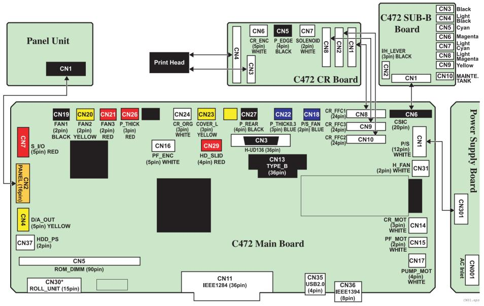
Figure 7-1. Stylus Pro 7600/9600 Connectors
