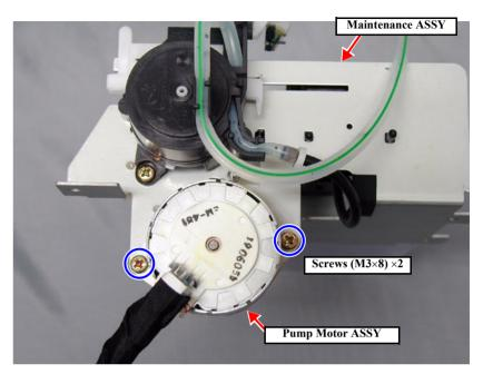
Figure 4-74. Removing the Pump Motor ASSY
