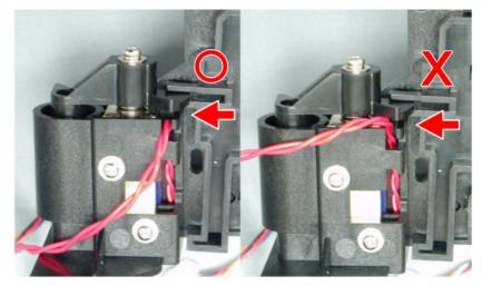
Figure 4-35. Take Care When Installing the Cutter Holder
