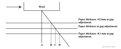
Figure 1-17. Displacement of Paper Thickness Detection Pattern
